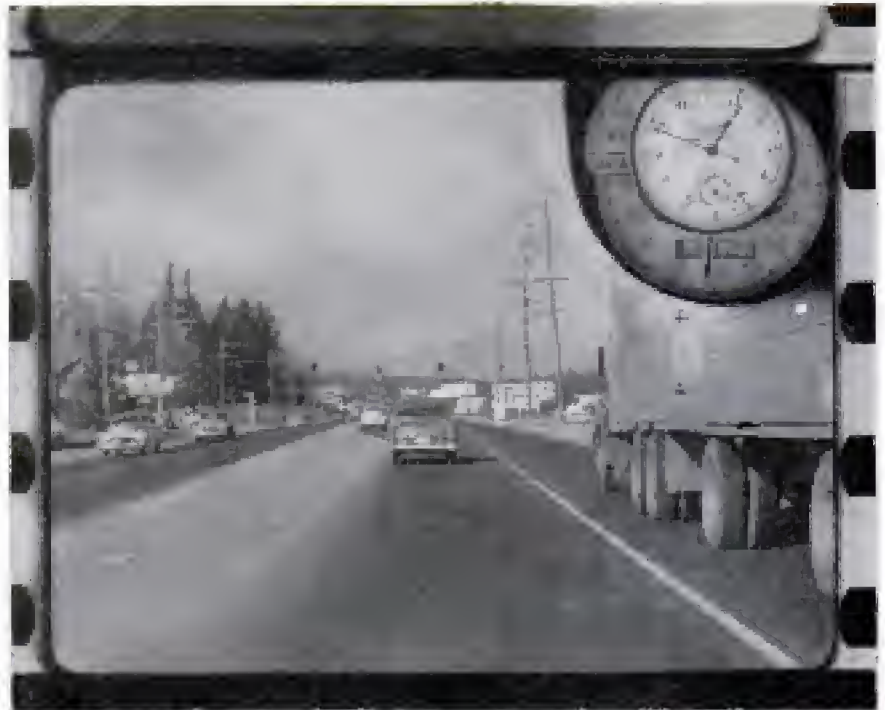
Frame from a film taken by the trafficamera shows car passing a truck and going 52 miles per hour. The camera automatically records the time and date also
